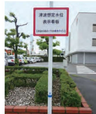
On-site indication of flood levels
